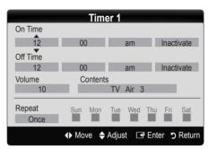
On Time / Off Time: Set the hour, minute, am/pm and activate / inactivate. (To activate the timer with the setting you have chosen, set to Activate.)
